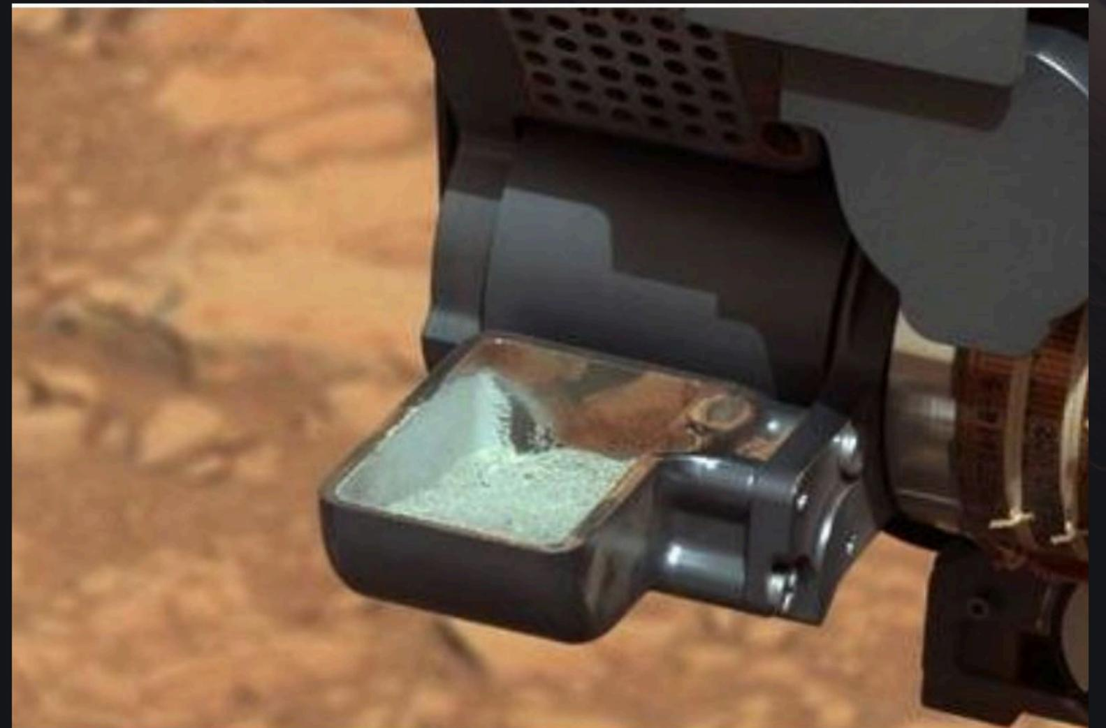
Drilling Sample in the Scoop
